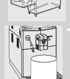
8 Place a large container (1.5 l) under both the steam/hot water wand and the dispensing spout.
