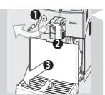
4 Insert the coffee grounds drawer back into the drip tray and this into the machine.
