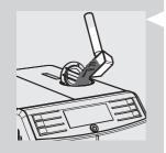
3 Lift the pre-ground coffee compartment lid and add one measuring scoop of pre-ground coffee to the compartment. Use only the measuring scoop supplied with the machine. Then close the pre-ground coffee compartment lid.
