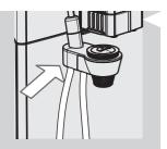
11 For storage you can put the suction tube as shown in the picture.
