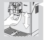
Move the dispensing spout up or down with your fingers to adjust its height as shown in the image.
