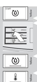
2 Press the "" button to start the cycle. The machine starts the automatic priming of the circuit by dispensing some water through the steam wand.
