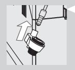
3 Insert the Automatic Milk Frother until it locks in place in the steam wand seat.
