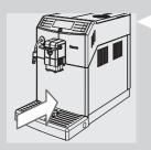
13 Insert the coffee grounds drawer with the drip tray back into the machine and close the service door.
