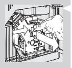
3 To remove the brew group, press the «PUSH» button pulling it by the handle and pull it out horizontally without turning it.
