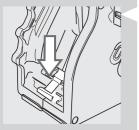
9 Gently pull down the lever until it is in contact with the brew group base and the two reference signs on the side of the brew group match.
