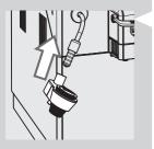
25 Remove the small white filter and replace the INTENZA+ water filter (if fitted) in the water tank. Reinsert the Automatic Milk Frother.
