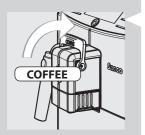
1 Push the lever upwards to select the "COFFEE" function.
