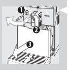
17 To clean the drip tray, place "Coffee Oil Remover" tablet inside and fill it 2/3rds full with hot water. Let the cleaning solution take effect for about 30 minutes, then rinse thoroughly.
