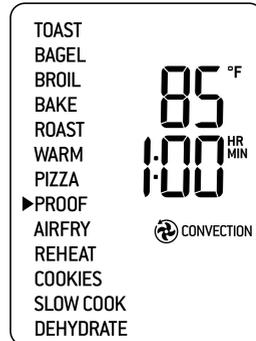
5. The proofing temperature, time and convection settings can be adjusted before or during the proof cycle.
