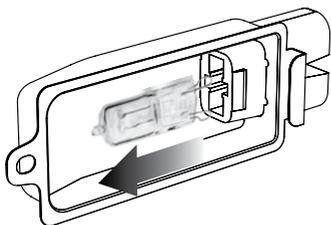
4. Use a soft cloth to insert the new bulb. Do not directly touch the surface of the bulb with your fingers as oil from your skin can damage the bulb.
