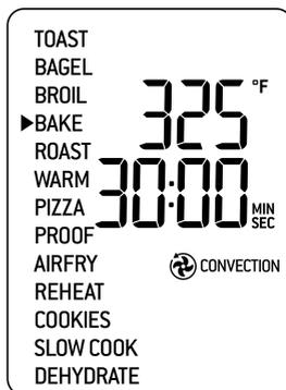
4. The baking temperature, time and convection settings can be adjusted before or during the baking cycle.
