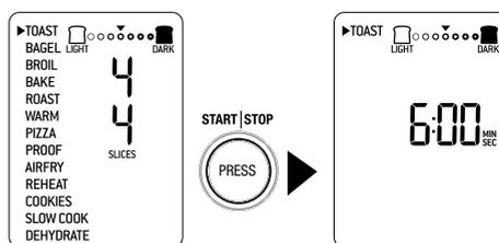
8. At the end of the TOAST cycle, the oven alert will sound. The START/STOP button backlight will go out and the LCD screen will illuminate white.
