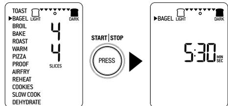
8. At the end of the BAGEL cycle, the oven alert will sound. The START/STOP button backlight will go out and the LCD screen will illuminate white.
