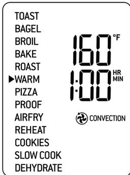
5. The temperature, time and convection settings can be adjusted before or during the warming cycle.
