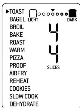
5. The darkness setting and number of slices can be adjusted before or during the toasting cycle.
