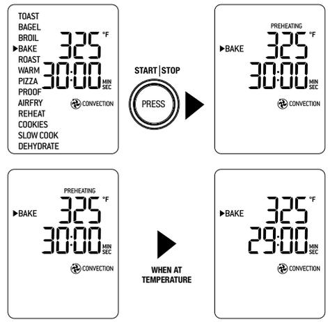
9. At the end of the BAKE cycle, the oven alert will sound. The START/STOP button backlight will go out and the LCD screen will illuminate white.
