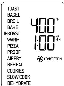
4. The roasting temperature, time and convection settings can be adjusted before or during the roasting cycle.
