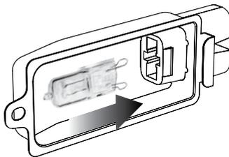
5. To reattach the glass cover, align the metal hook with the left side of the light housing. Slide the opposite end of the glass cover into the metal bracket on the right side of the housing, then push the metal hook into the left side of the housing until it snaps securely into position.
