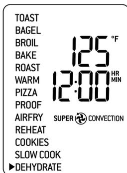
4. The dehydrating temperature, time and convection settings can be adjusted before or during the dehydrate cycle.
