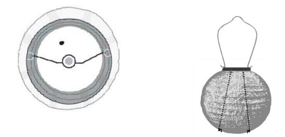
**Step Three:** Attach the wire hanging handle by inserting the curved ends of the handle into the raised tabs located on the top of the plastic solar housing compartment. The molded tabs are designed with a small hole through which the curved end of the wire hanging handle will easily fit. Attach both sides of the wire hanging handle. The solar panel must be facing upwards towards the sun in order to be able to collect sunlight.
